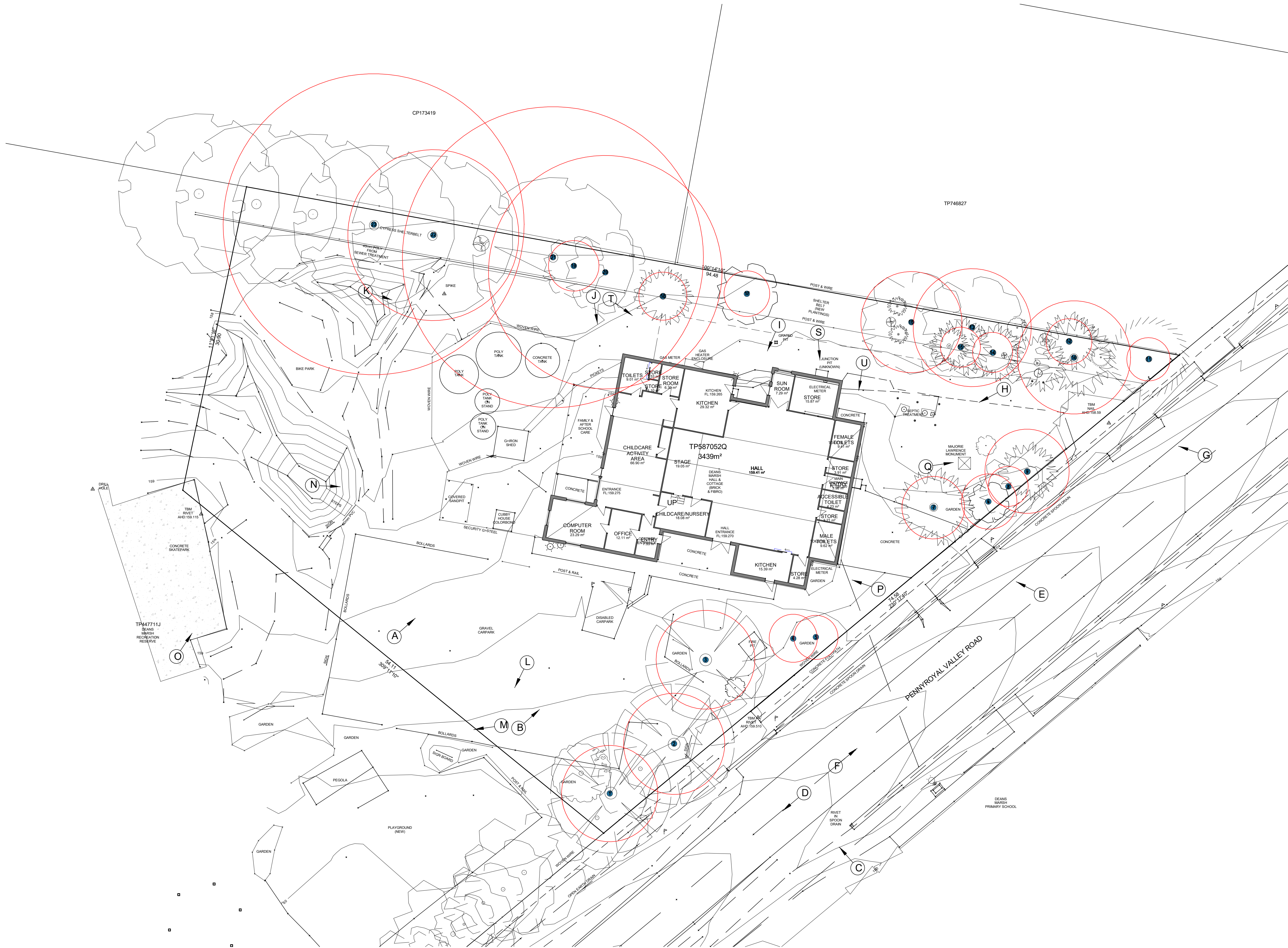
1 EXISTING SITE SURVEY WITH BUILDING PLAN 1 : 200
