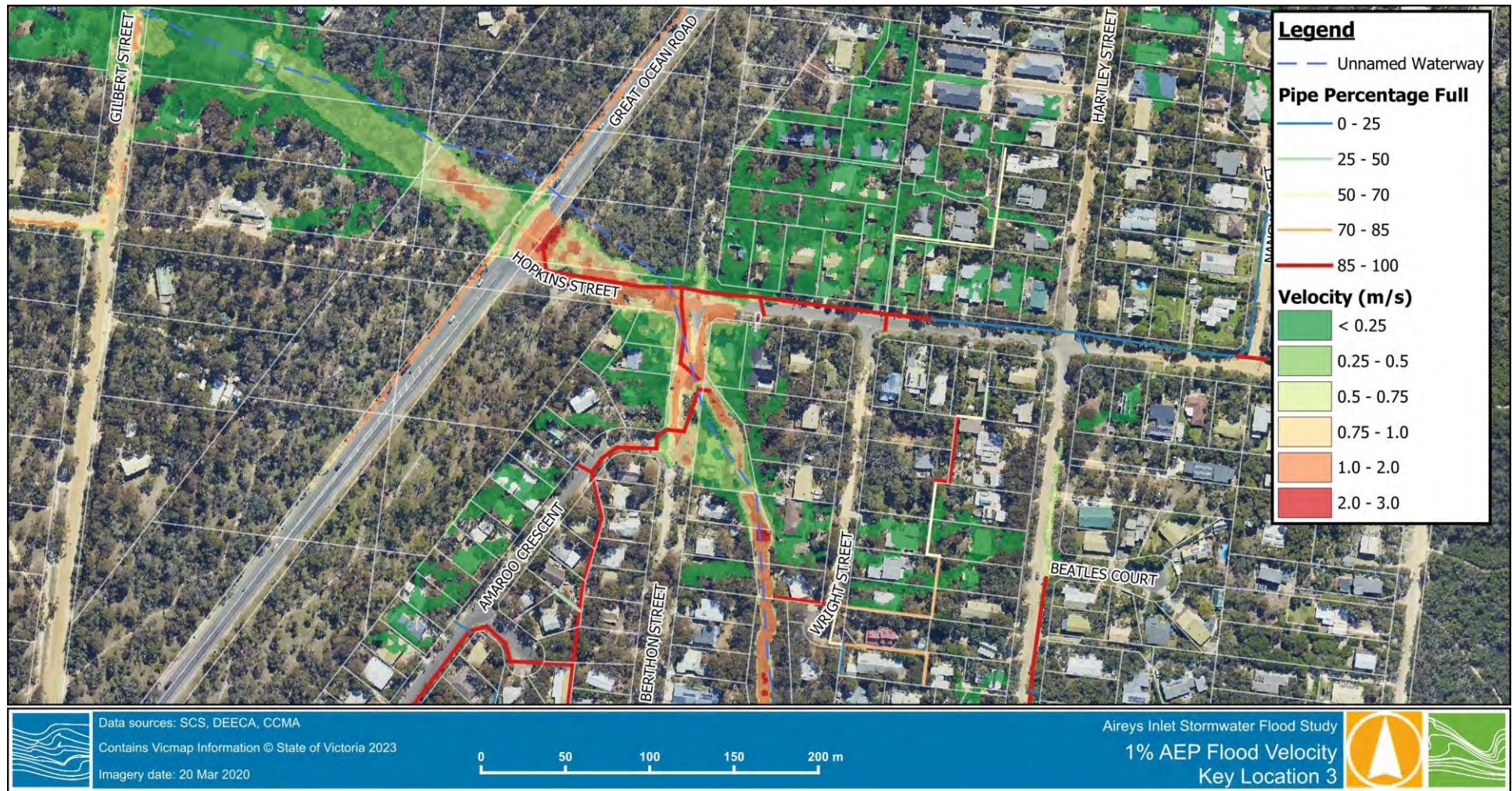
Figure 3-9 1% AEP Flood Velocity – Key Location 3
