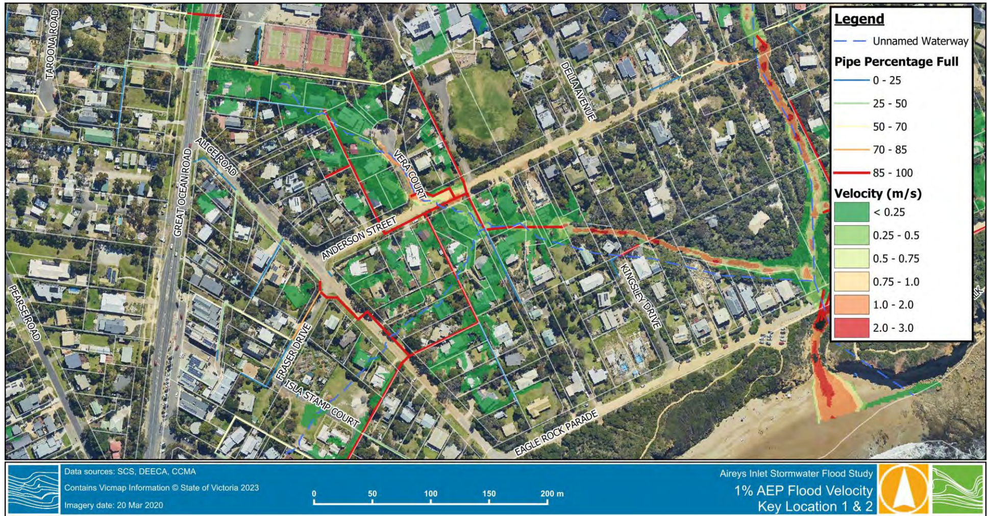
Figure 3-5 1% AEP Flood Velocity – Key Location 1
