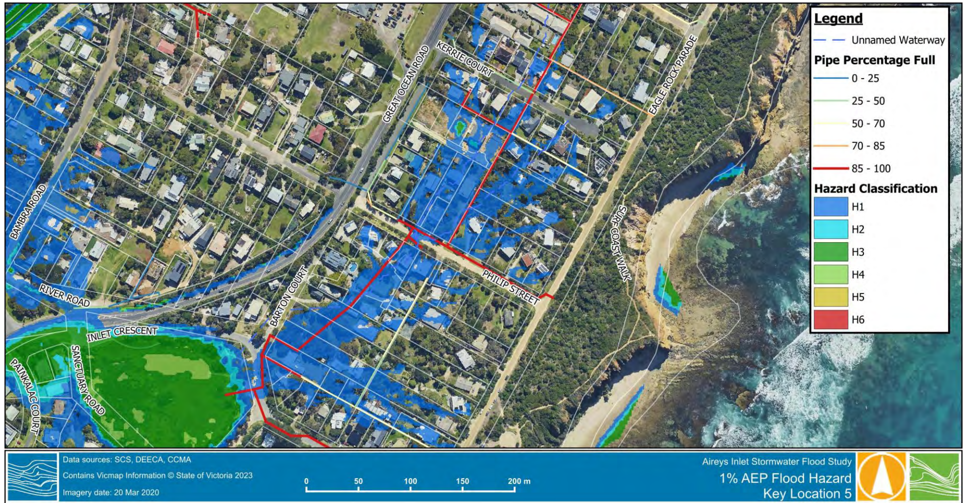
Figure 3-19 1% AEP Flood Hazard – Key Location 5
