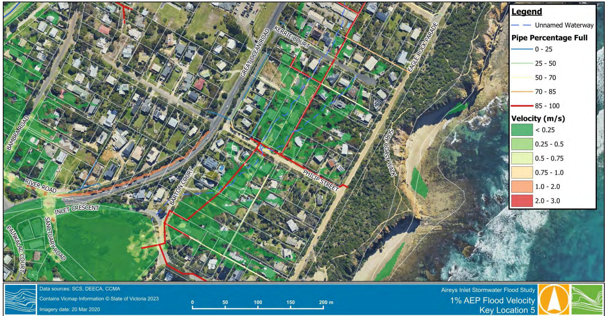
Figure 3-17 1% AEP Flood Velocity – Key Location 5
