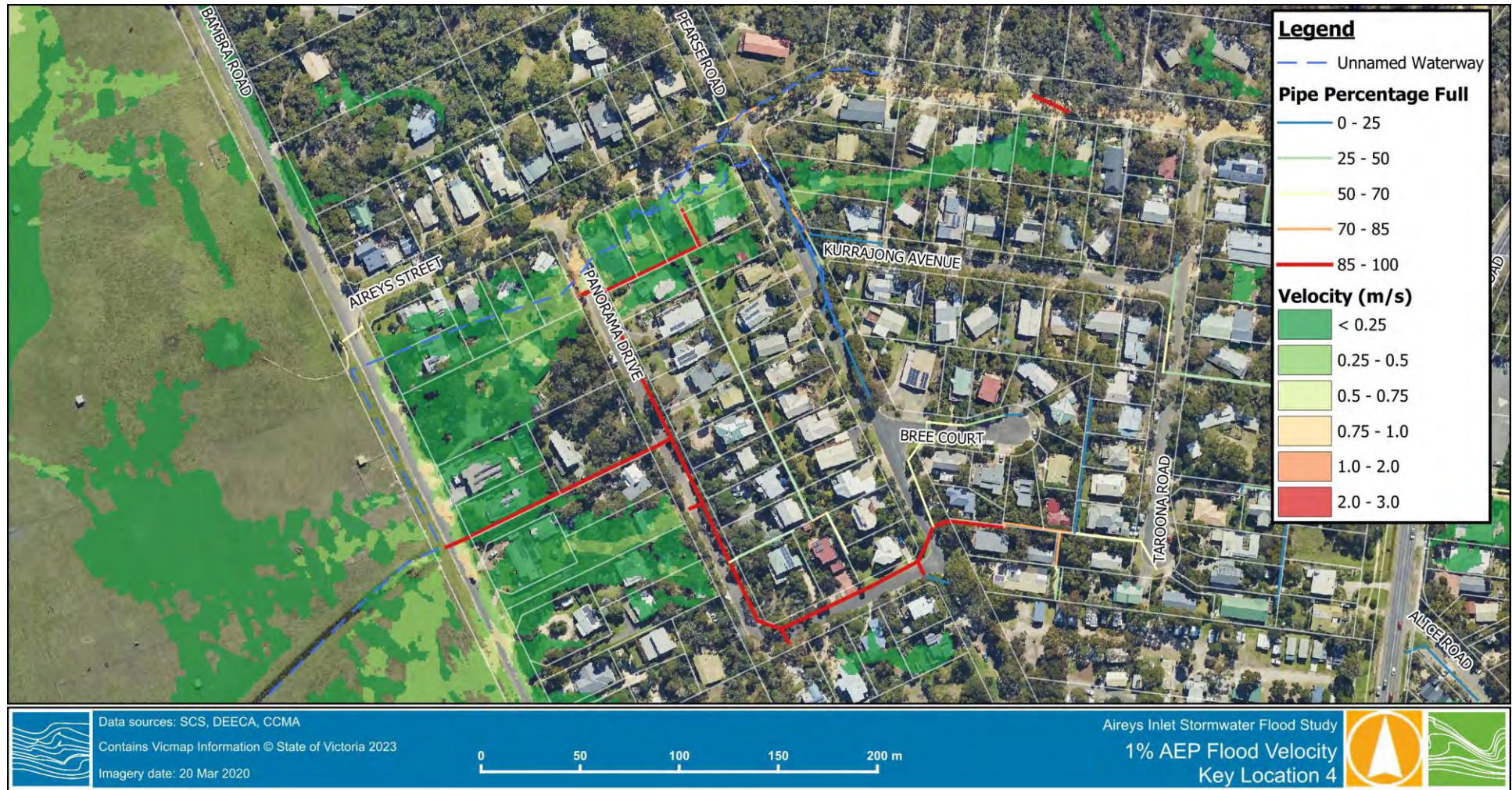
Figure 3-13 1% AEP Flood Velocity – Key Location 4
