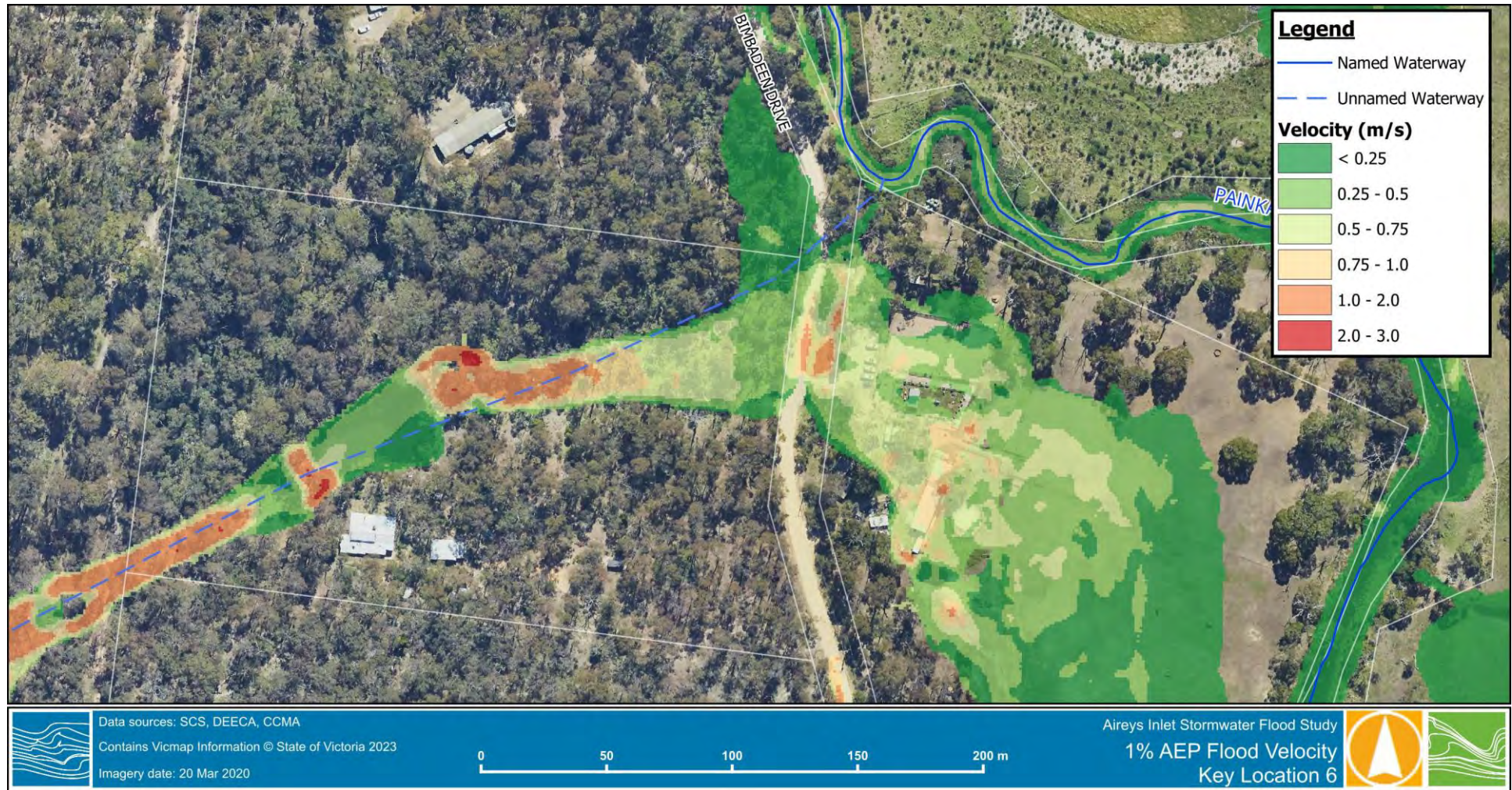
Figure 3-21 1% AEP Flood Velocity – Key Location 6
