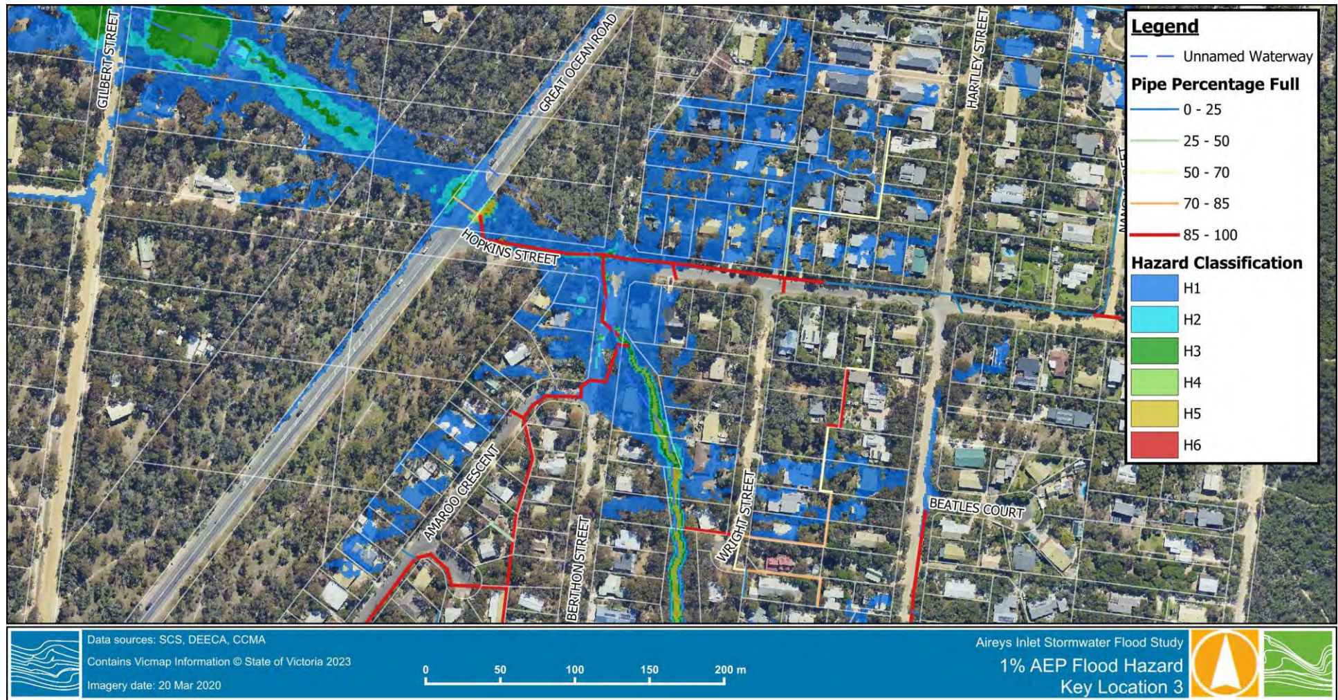
Figure 3-11 1% AEP Flood Hazard – Key Location 3
