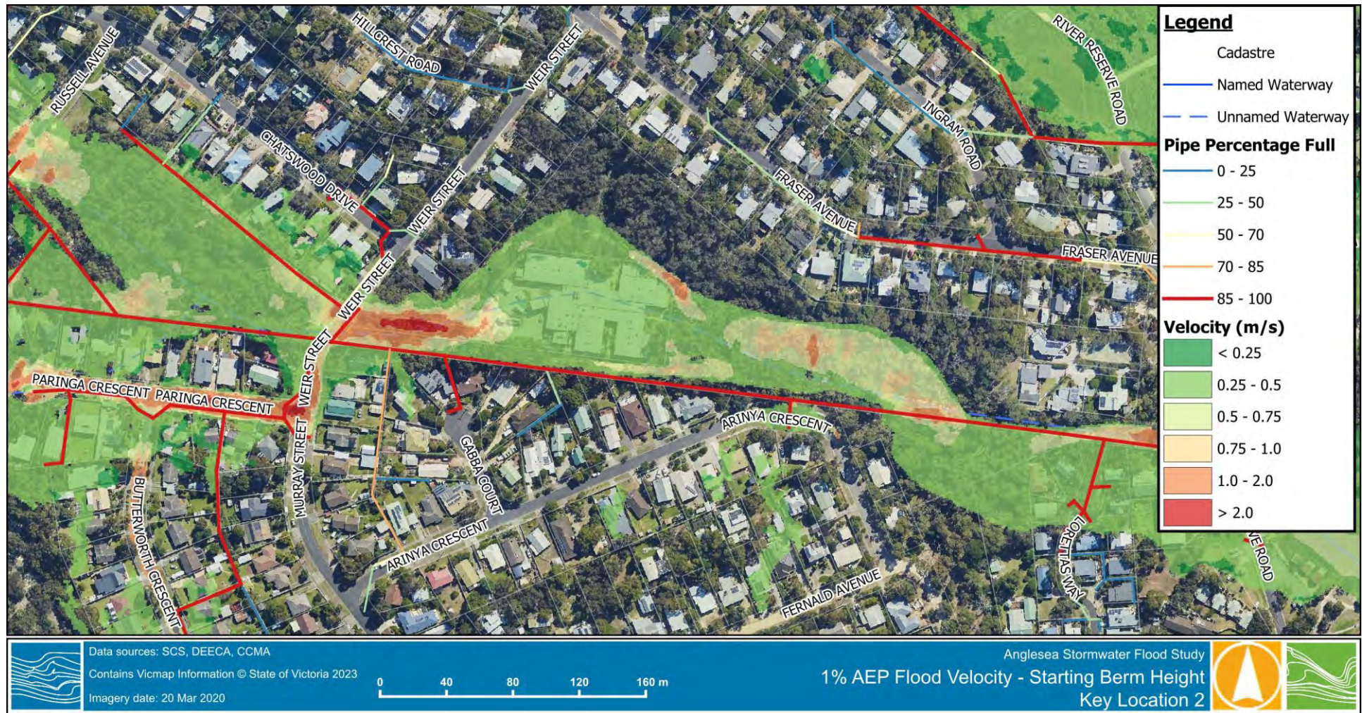
Figure 3-10 1% AEP Flood Velocity – Key Location 2
