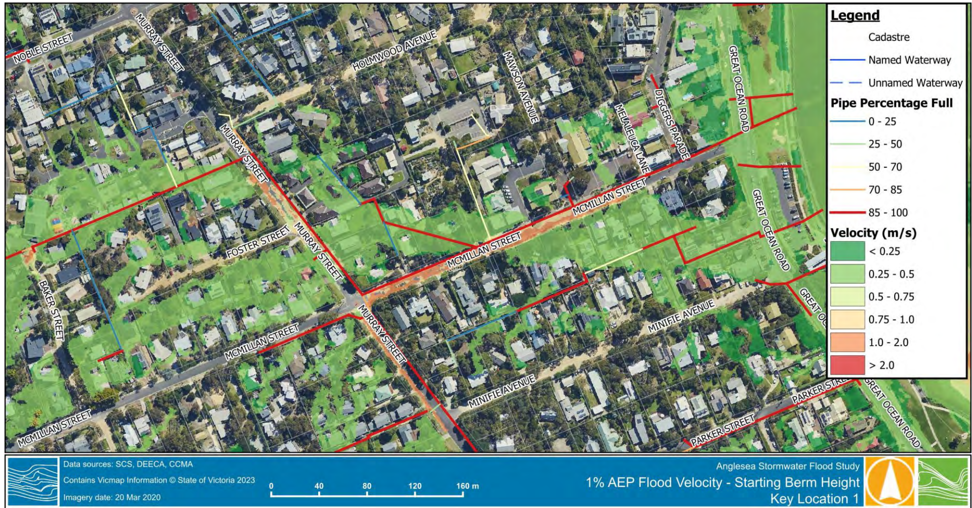
Figure 3-6 1% AEP Flood Velocity – Key Location 1
