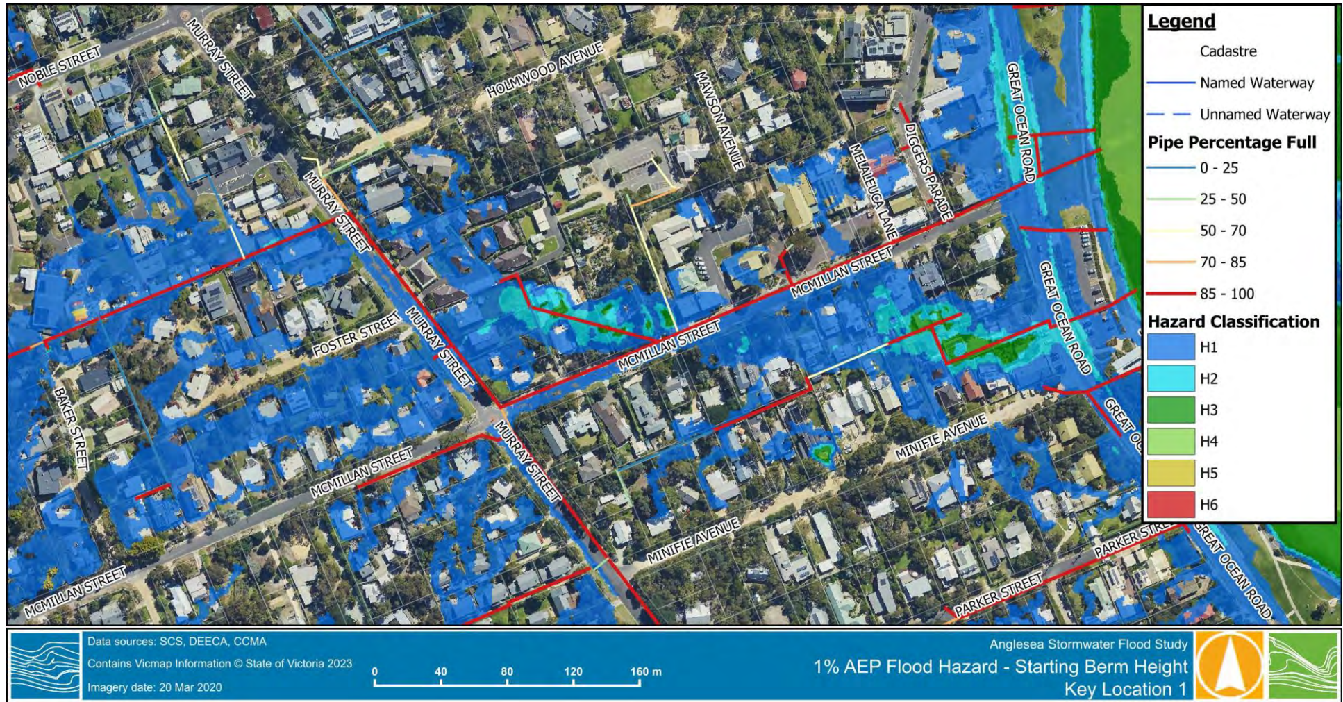
Figure 3-8 1% AEP Flood Hazard – Key Location 1
