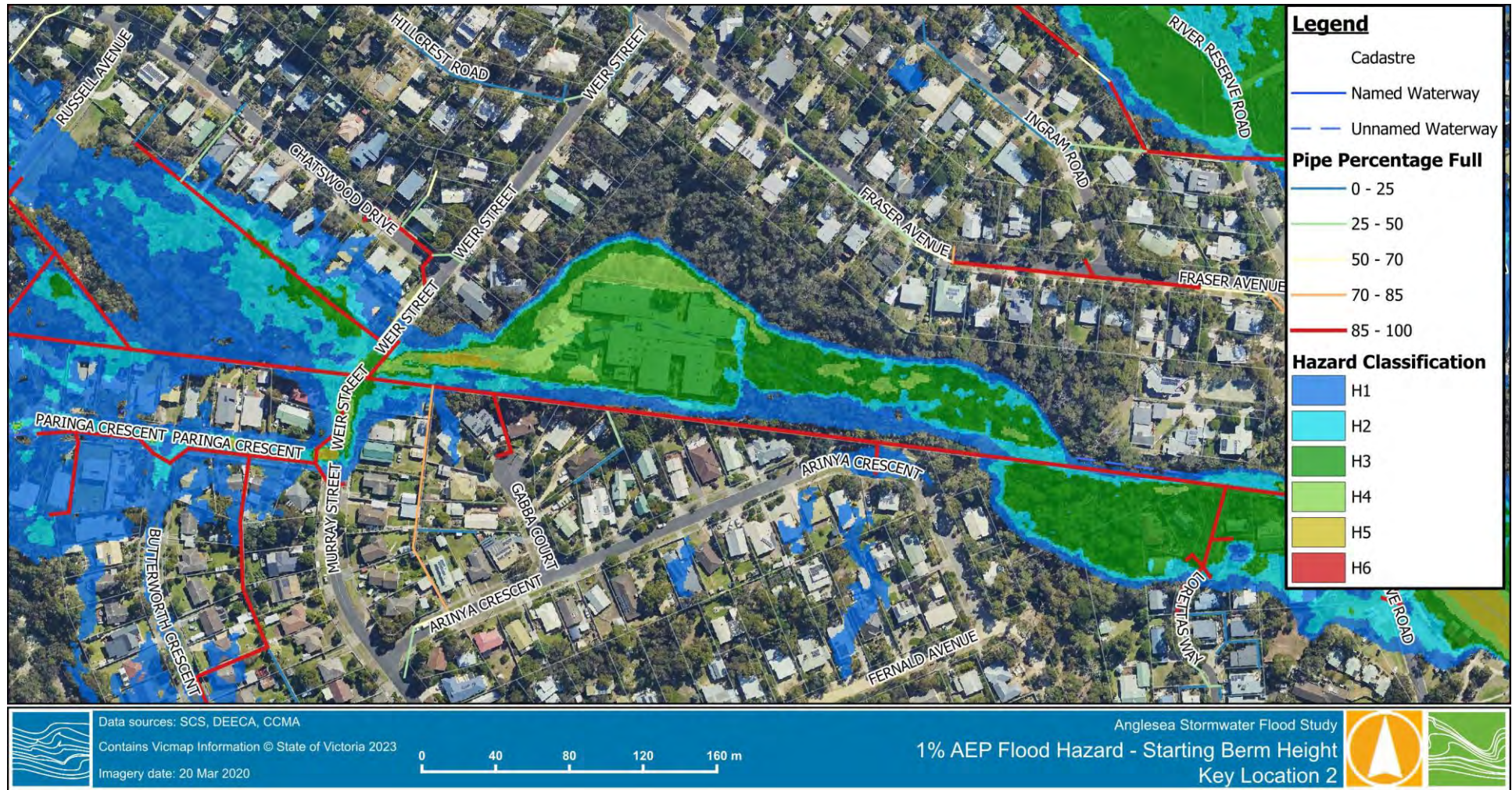
Figure 3-12 1% AEP Flood Hazard – Key Location 2
