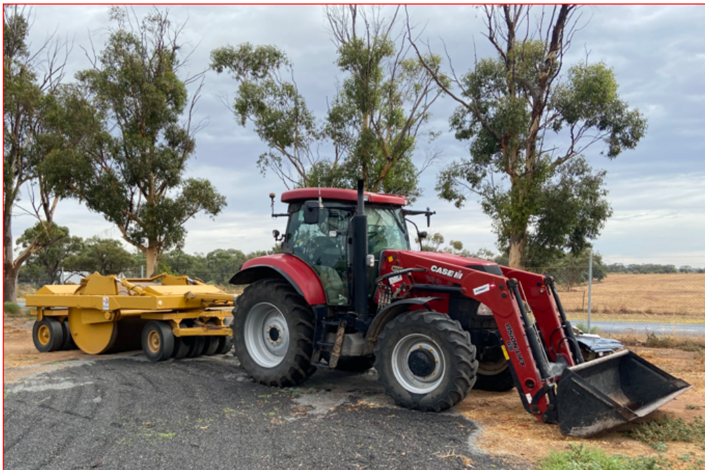
Figure 18: (example) Tractor Drawn Combination Multi-Tyred and Steel Drum Roller Unit
